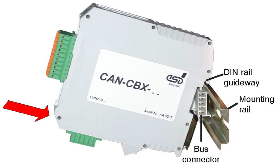
Figure 6 : Mounting CAN-CBX modules
