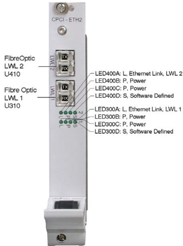
Fig. 3.3.1: Position of the LEDs and connectors of the CPCI-ETH2-FX
