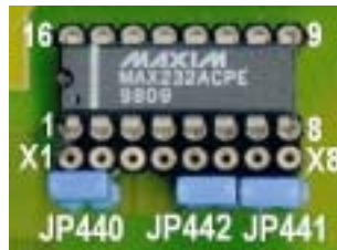
Fig. 2.2.2: Position of the RS-232 driver and the piggybacks at the plug-in place
