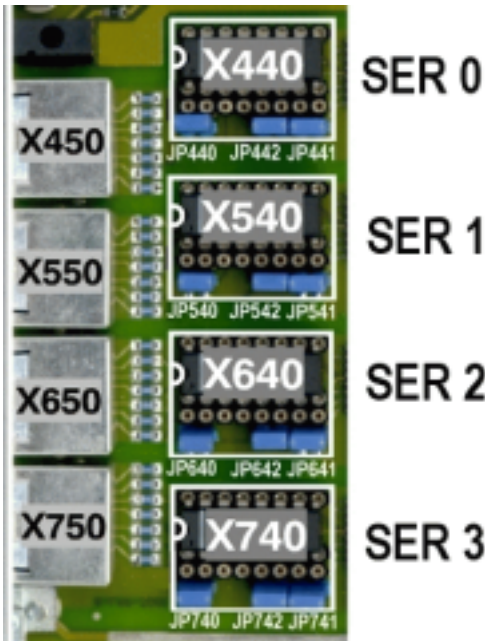
Fig. 2.2.3: Assignment of the plug-in places to the serial channels (shown example: RS-232 mode)
