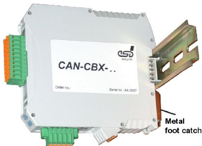
Figure. 33: Mounted CAN-CBX module
