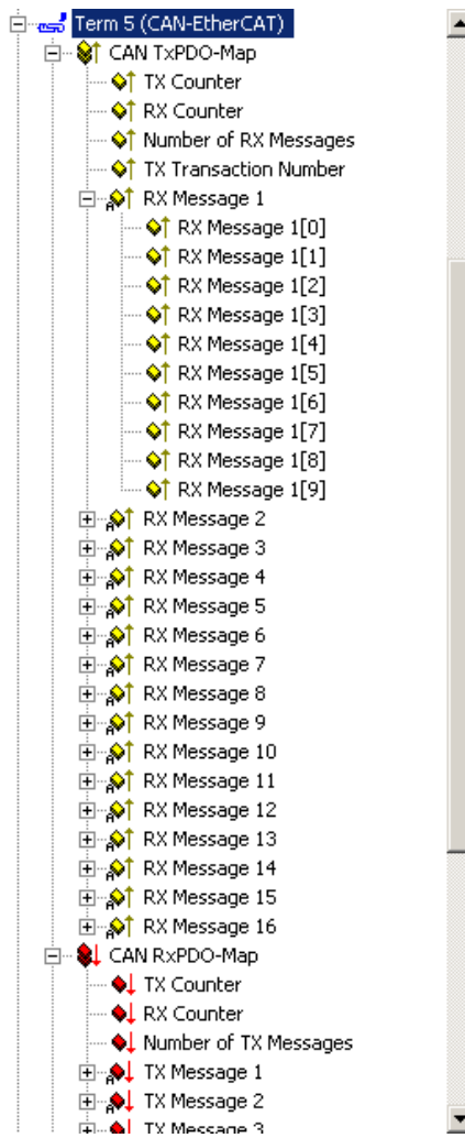
Figure 14: Can interface process image
